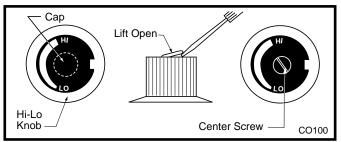
Fig. 58 Remove center screw from Hi-Lo knob.
